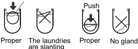
(2) Close the inner and outer cover of the spin tub.
